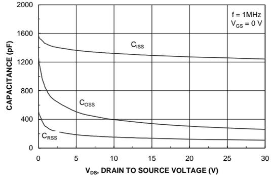
Figure 8. Capacitance Characteristics.
