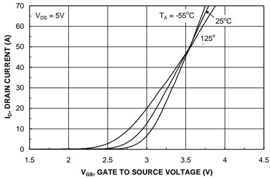
Figure 5. Transfer Characteristics.
