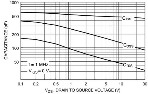
Figure 8. Capacitance Characteristics.
