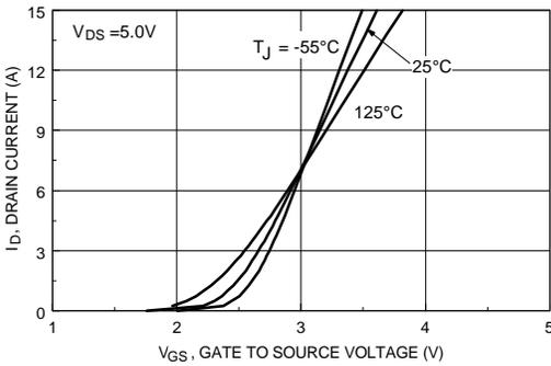
Figure 5. Transfer Characteristics.
