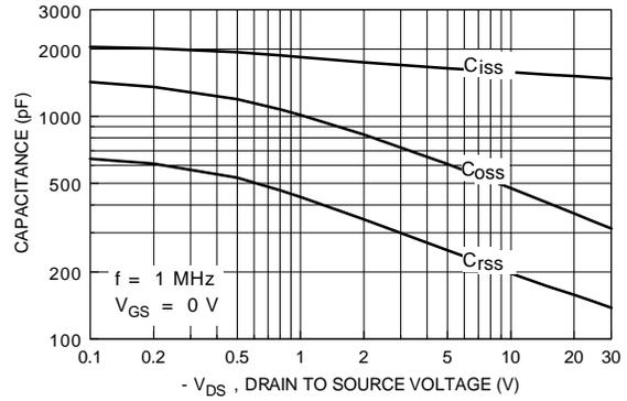
Figure 8. Capacitance Characteristics.
