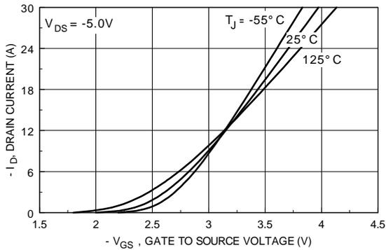
Figure 5. Transfer Characteristics.
