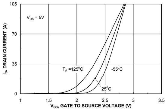
Figure 5. Transfer Characteristics.
