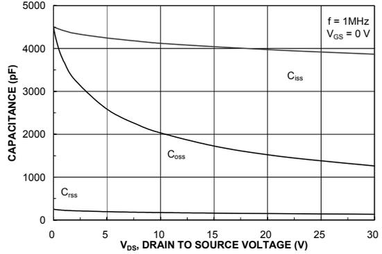
**Figure 8. Capacitance Characteristics.**
