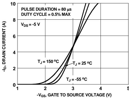
**Figure 5. Transfer Characteristics**
