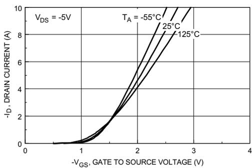
**Figure 5. Transfer Characteristics.**
