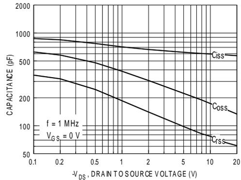
**Figure 8. Capacitance Characteristics.**
