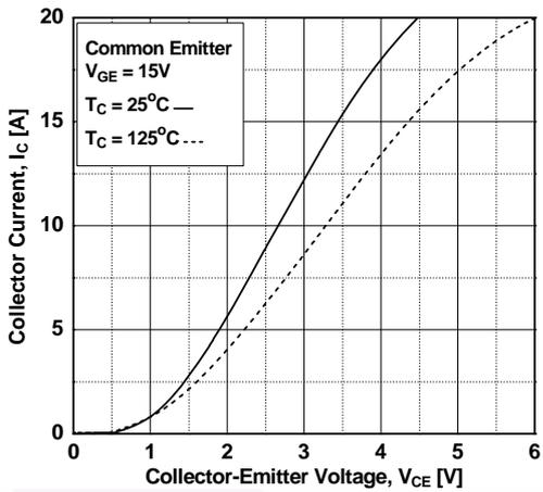
Figure 4. Transfer Characteristics
