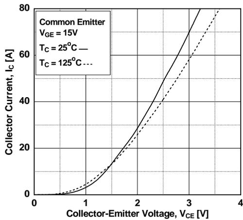
**Figure 4. Transfer Characteristics**
