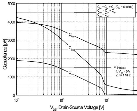
Figure 5. Capacitance Characteristics
