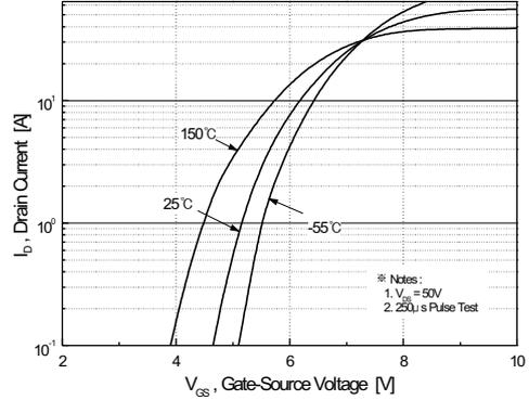
Figure 2. Transfer Characteristics
