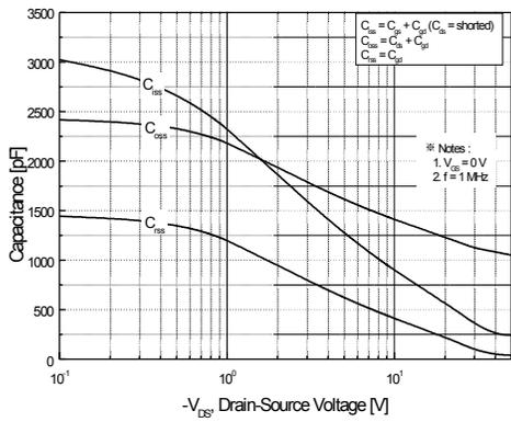
Figure 5. Capacitance Characteristics
