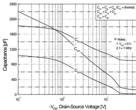
**Figure 5. Capacitance Characteristics**
