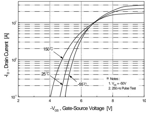
**Figure 2. Transfer Characteristics**
