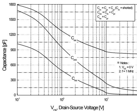
Figure 5. Capacitance Characteristics
