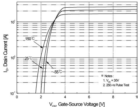
Figure 2. Transfer Characteristics
