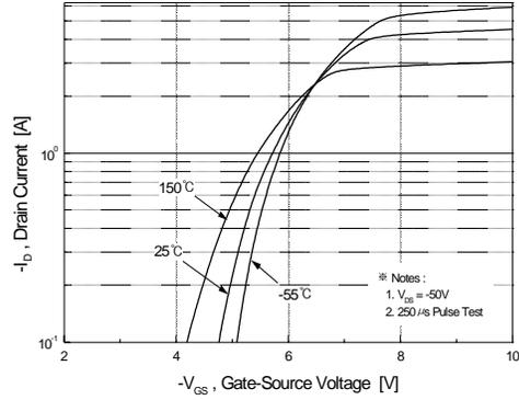
Figure 2. Transfer Characteristics
