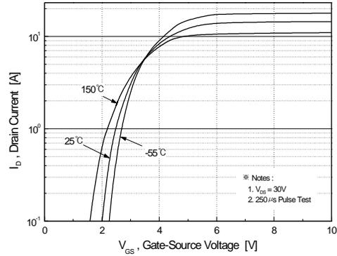
**Figure 2. Transfer Characteristics**
