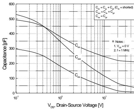
**Figure 5. Capacitance Characteristics**
