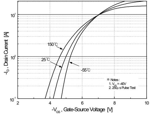
Figure 2. Transfer Characteristics
