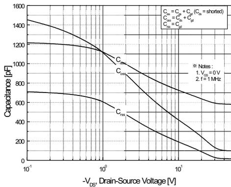
Figure 5. Capacitance Characteristics
