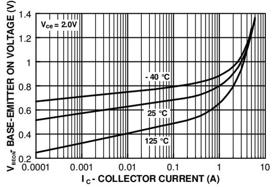
Figure 2. Base-Emitter On Voltage vs Collector Current
