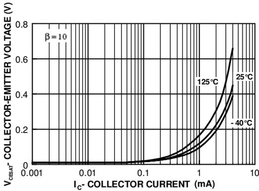
Figure 3. Collector-Emitter Saturation Voltage vs Collector Current
