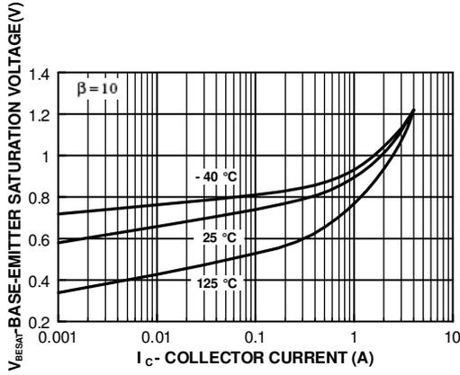
Figure 1. Base-Emitter Saturation Voltage vs Collector Current
