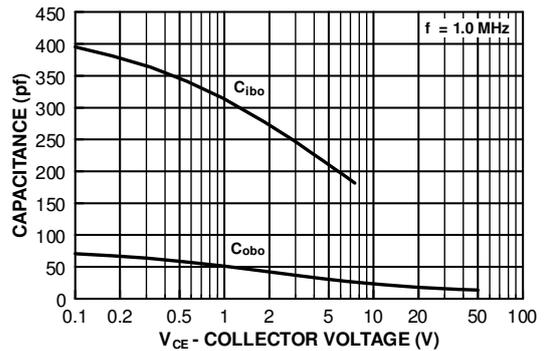
Figure 4. Input/Output Capacitance vs Reverse Bias Voltage
