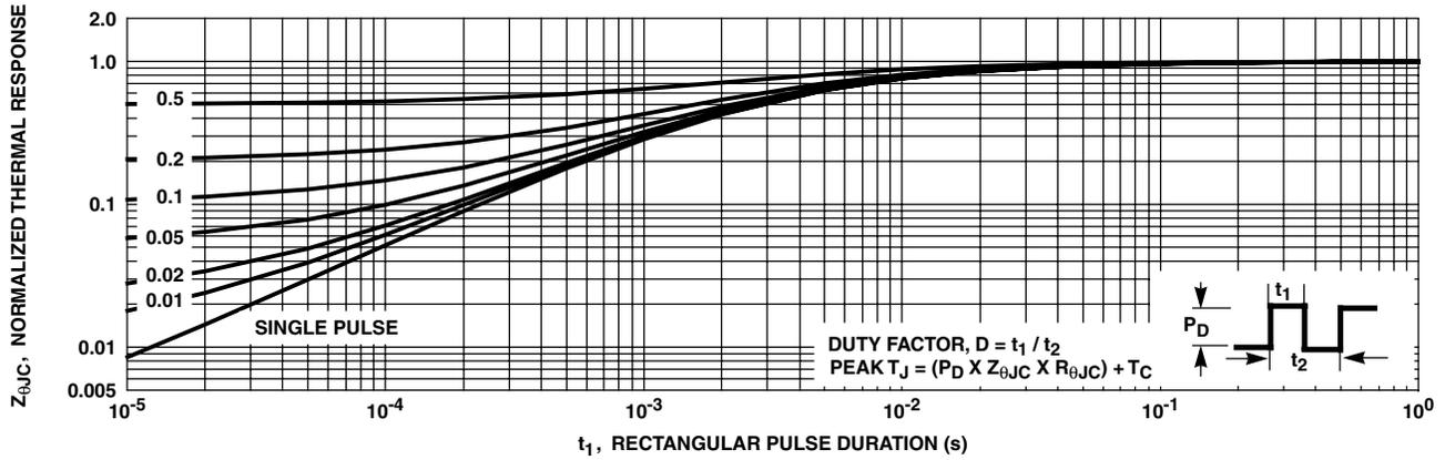
FIGURE 17. NORMALIZED TRANSIENT THERMAL RESPONSE, JUNCTION TO CASE
