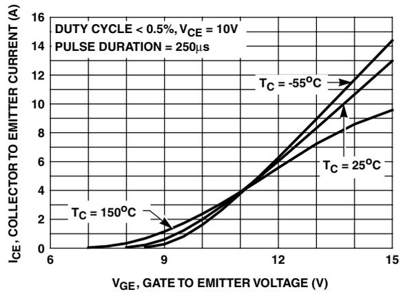
FIGURE 13. TRANSFER CHARACTERISTIC
