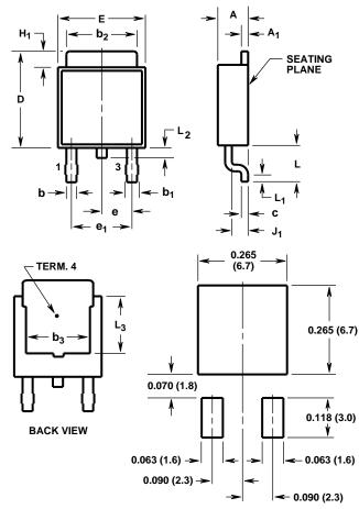
MINIMUM PAD SIZE RECOMMENDED FOR SURFACE-MOUNTED APPLICATIONS
