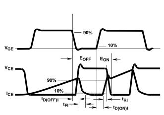
FIGURE 19. SWITCHING TEST WAVEFORMS
