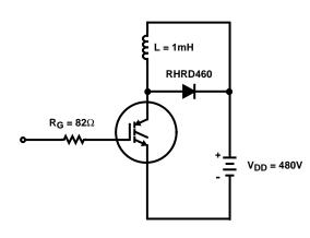
FIGURE 18. INDUCTIVE SWITCHING TEST CIRCUIT
