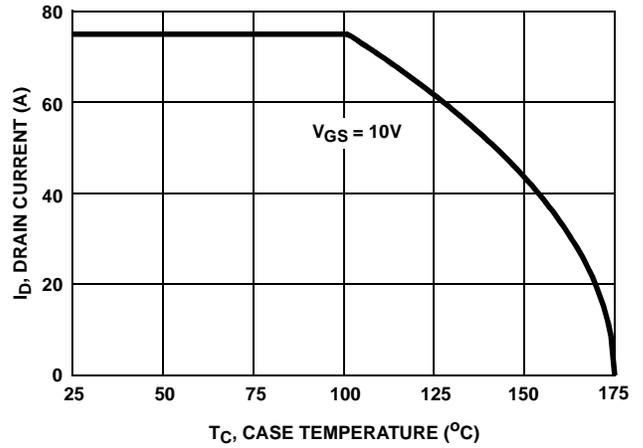
FIGURE 2. MAXIMUM CONTINUOUS DRAIN CURRENT vs CASE TEMPERATURE
