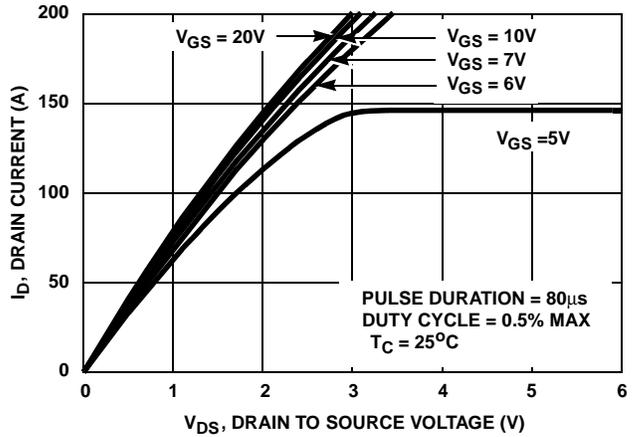
FIGURE 8. SATURATION CHARACTERISTICS
