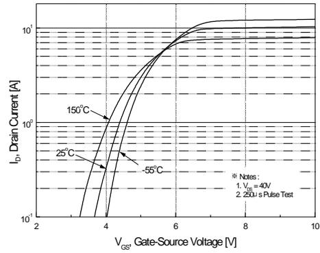
Figure 2. Transfer Characteristics
