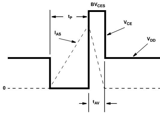
Figure 20. Energy Waveforms
