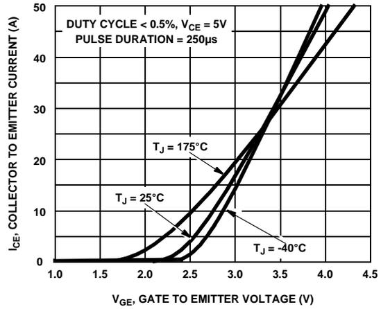
Figure 8. Transfer Characteristics
