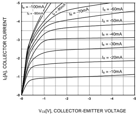
Figure 1. Static Characteristic
