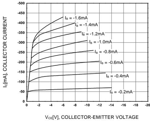
Figure 1. Static Characteristic
