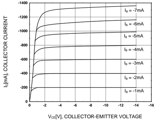
Figure 1. Static Characteristic
