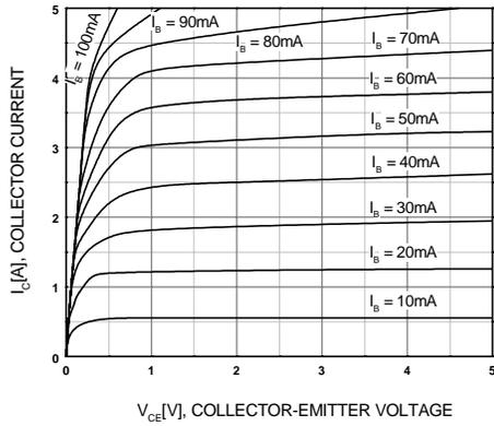
Figure 1. Static Characteristic
