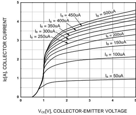
Figure 1. Static Characteristic
