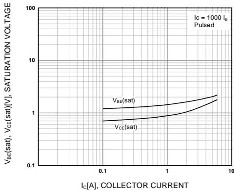
Figure 3. Collector-Emitter Saturation Voltage Base-Emitter Saturation Voltage
