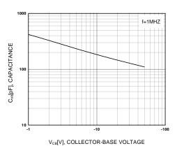
Figure 3. Collector Output Capacitance
