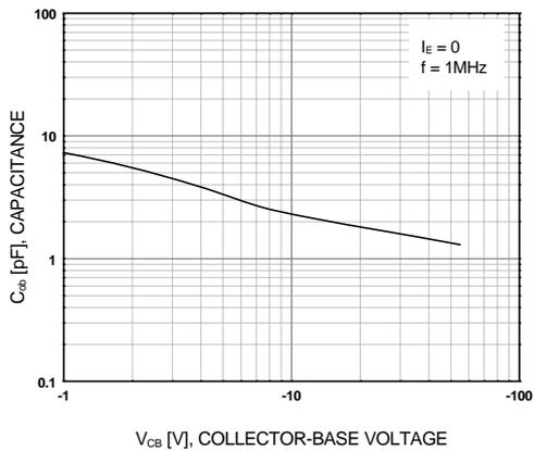
Figure 3. Output Capacitance
