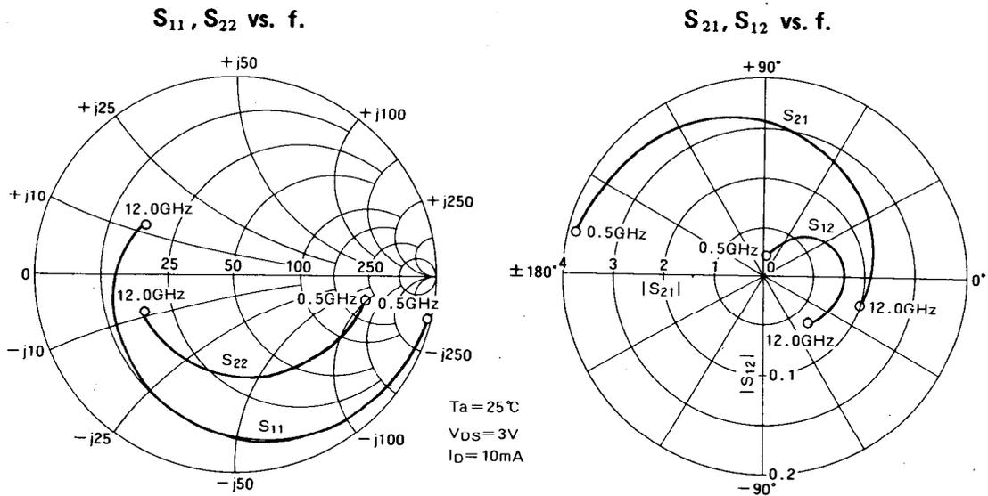
**S PARAMETERS** ( $T_a = 25^\circ\text{C}$ ,  $V_{DS} = 3\text{V}$ ,  $I_D = 10\text{mA}$ )
