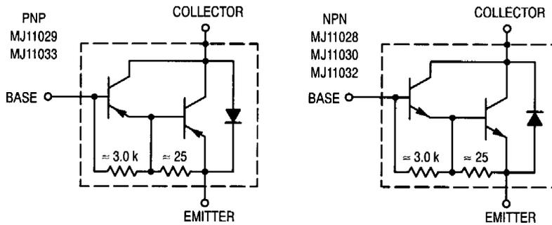
Figure 1. Darlingon Circuit Schematic
