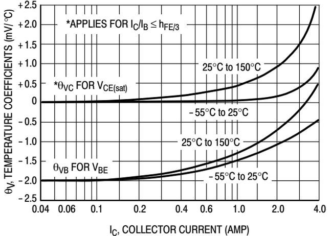
**Figure 6. Temperature Coefficients**
