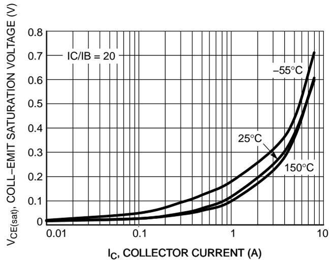
Figure 9. MJD45H11 Saturation Voltage
