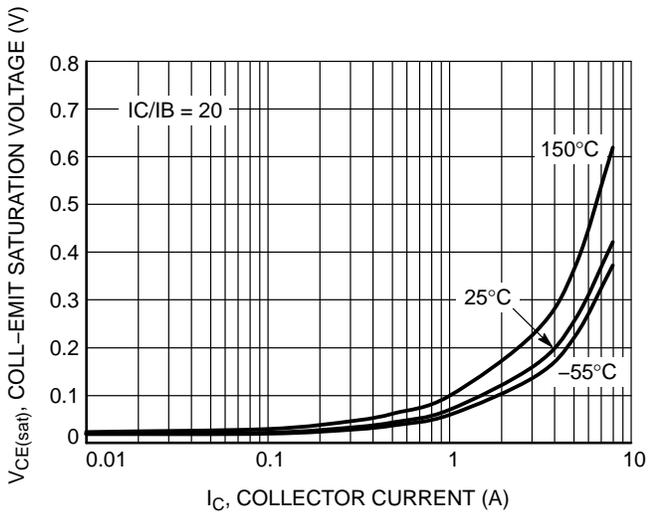
Figure 8. MJD44H11 Saturation Voltage
