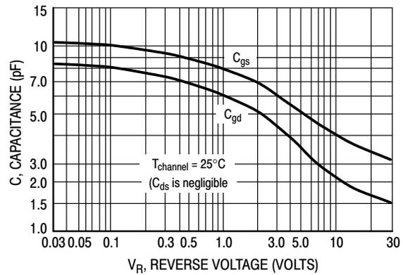
Figure 7. Typical Capacitance
