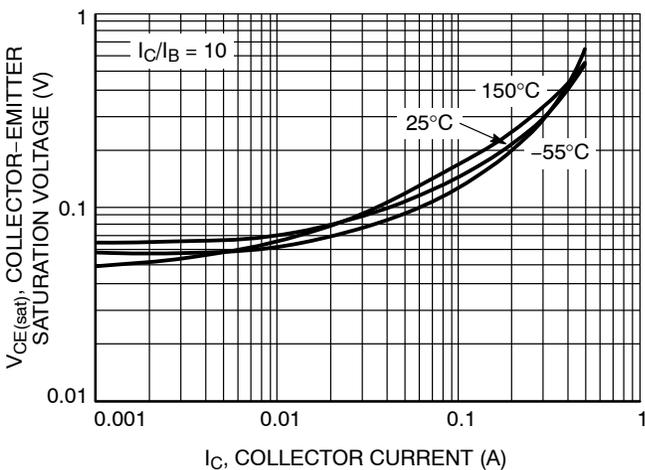
Figure 11. Collector-Emitter Saturation Voltage vs. Collector Current
