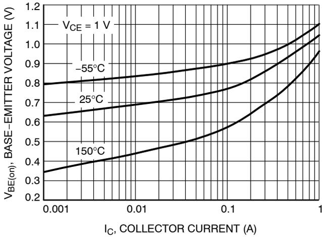
**Figure 13. Base Emitter Voltage vs. Collector Current**
