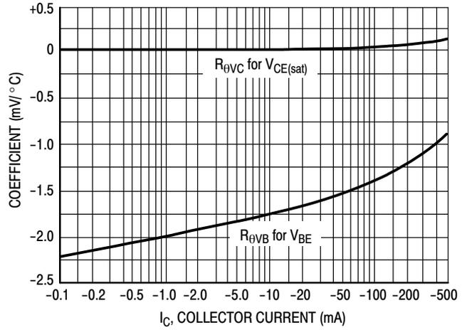
**Figure 14. Temperature Coefficients**
