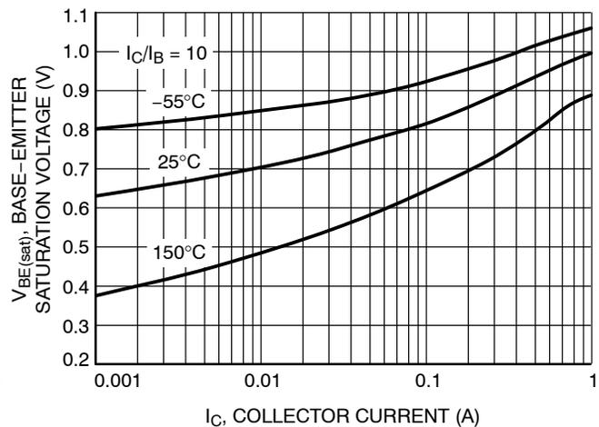
Figure 12. Base-Emitter Saturation Voltage vs. Collector Current
