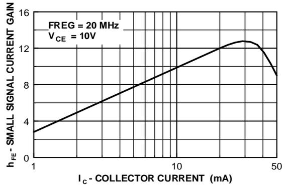
Figure 8. Small Signal Current Gain vs Collector Current
