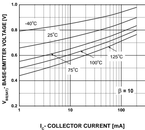
Figure 3. Base-Emitter Saturation Voltage vs Collector Current
