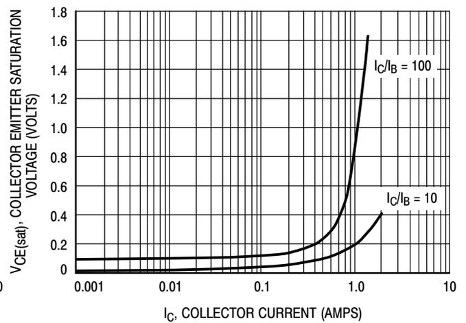
**Figure 6. Collector Emitter Saturation Voltage versus Collector Current**
