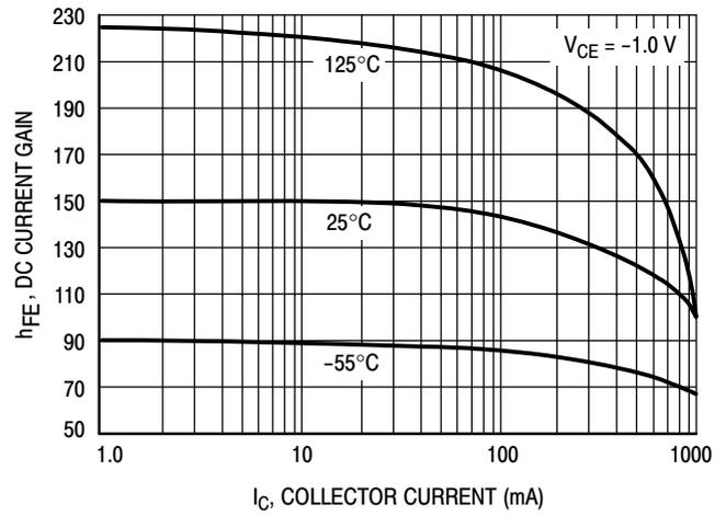
**Figure 2. DC Current Gain versus Collector Current**
