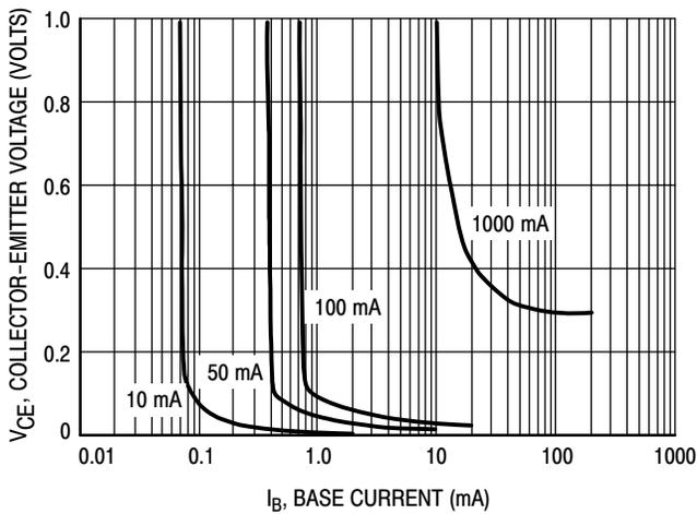
**Figure 5. Collector Emitter Saturation Voltage versus Collector Current**
