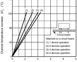
Total power dissipation P<sub>T</sub> (W)
