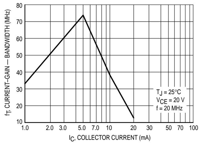
Figure 3. Current-Gain - Bandwidth
