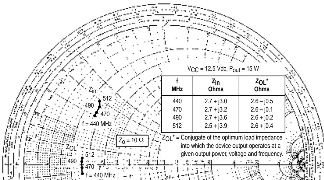
Figure 6. Series Equivalent Input and Output Impedance
