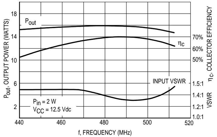
Figure 5. Typical Broadband Circuit Performance
