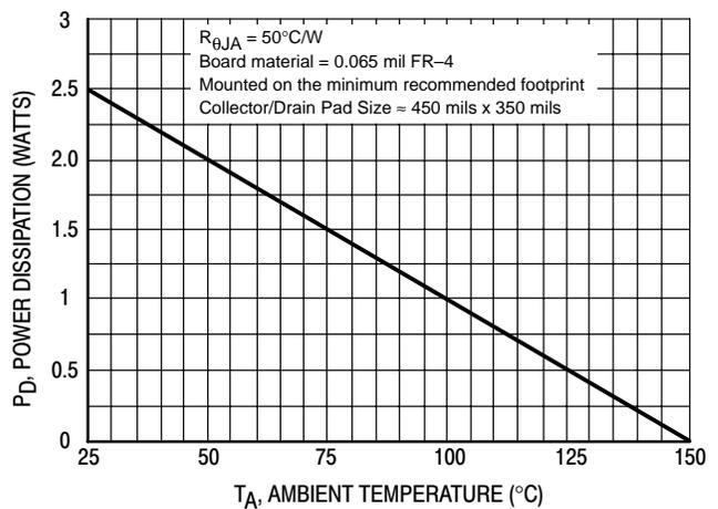
Figure 15. D<sup>2</sup>PAK Power Derating Curve
