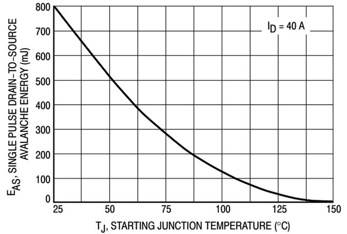
Figure 12. Maximum Avalanche Energy versus Starting Junction Temperature
