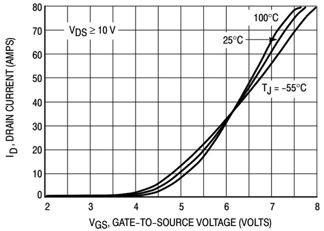
Figure 2. Transfer Characteristics
