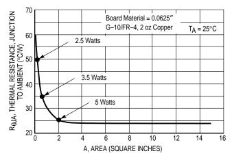
Figure 16. Thermal Resistance versus Drain Pad Area for the D<sup>2</sup>PAK Package (Typical)
