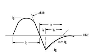
Figure 14. Diode Reverse Recovery Waveform
