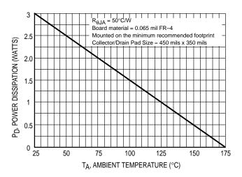
Figure 15. D<sup>2</sup>PAK Power Derating Curve
