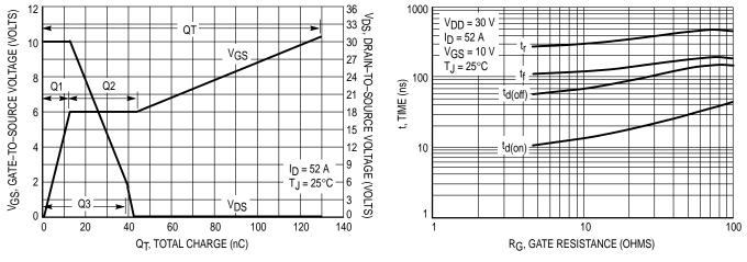
Figure 8. Gate–To–Source and Drain–To–Source Voltage versus Total Charge
