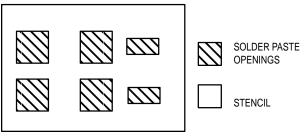
Figure 17. Typical Stencil for DPAK and D<sup>2</sup>PAK Packages
