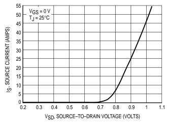
Figure 10. Diode Forward Voltage versus Current
