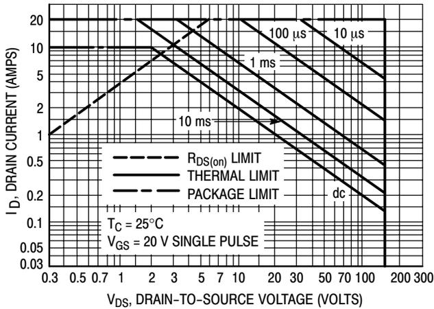
Figure 8. Maximum Rated Forward Biased Safe Operating Area
