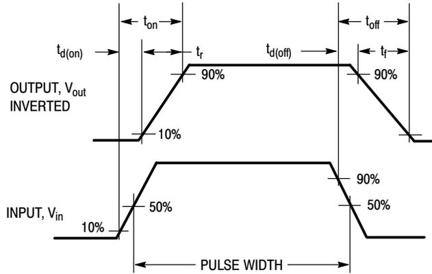
Figure 14. Switching Waveforms
