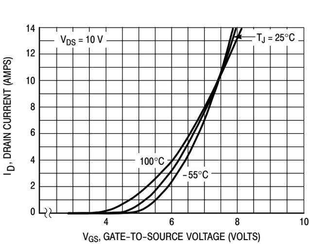
Figure 4. Transfer Characteristics
