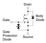
Remark The diode connected between the gate and source of the transistor serves as a protector against ESD. When this device actually used, an additional protection circuit is externally required if a voltage exceeding the rated voltage may be applied to this device.
