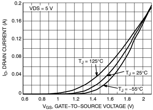
Figure 2. Transfer Characteristics
