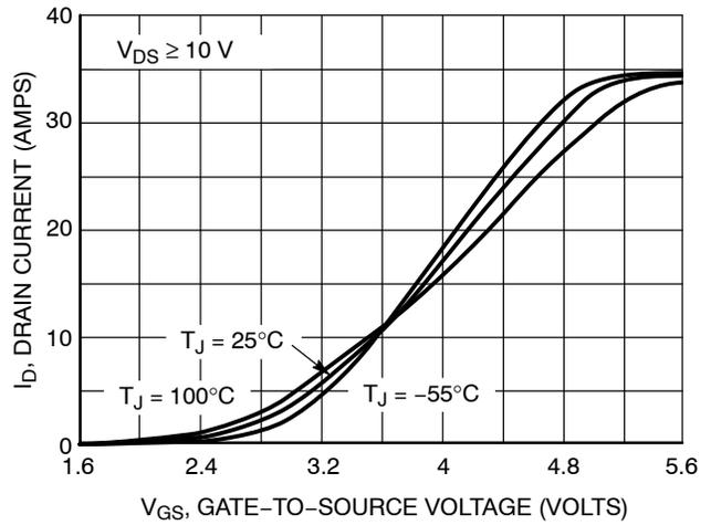
**Figure 2. Transfer Characteristics**
