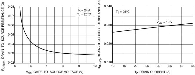
Figure 3. On-Resistance vs. Gate-to-Source Voltage
