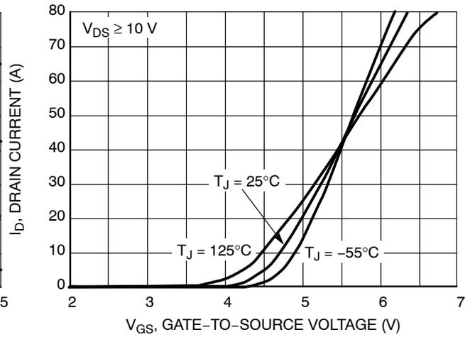
Figure 2. Transfer Characteristics
