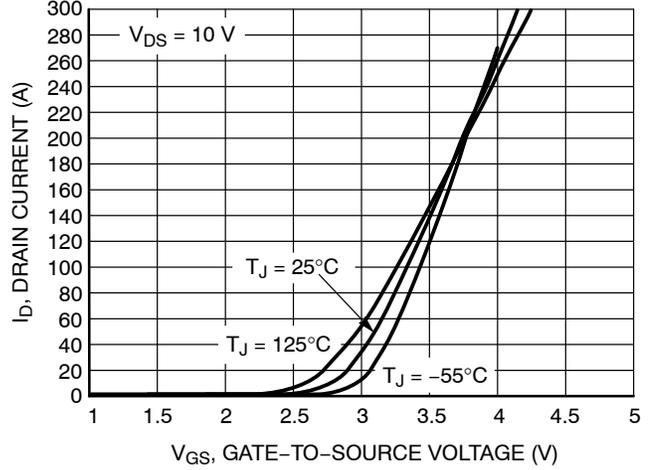
Figure 2. Transfer Characteristics
