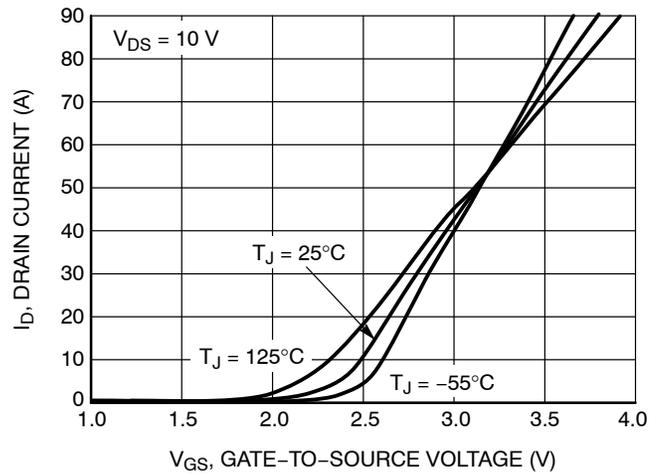
Figure 2. Transfer Characteristics
