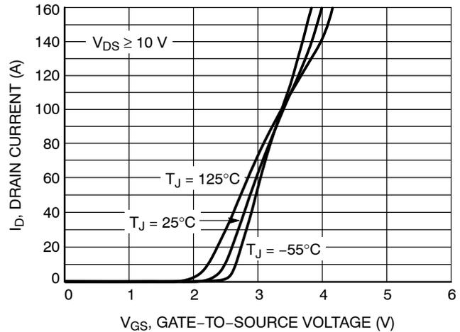
Figure 2. Transfer Characteristics
